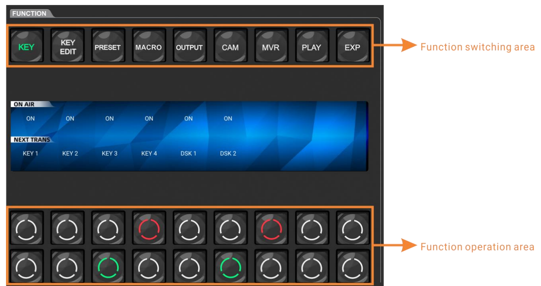
Figure 5-9 Comprehensive control area
