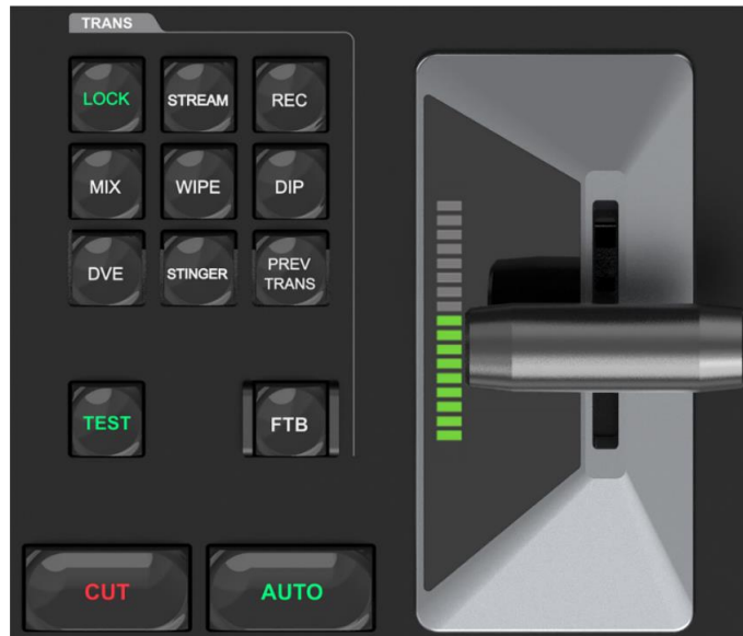
Figure 5-19 Transition control area
