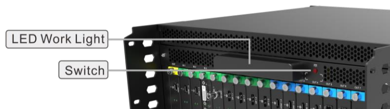
Figure 5-3 Rear panel LED work lights
