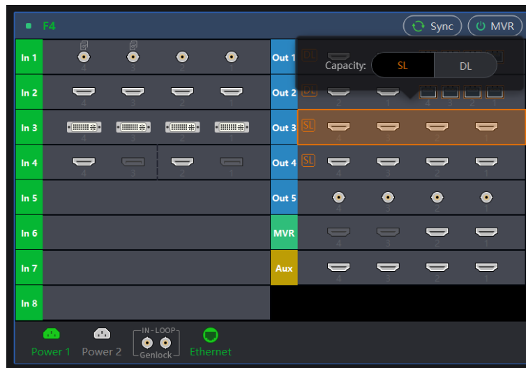
Figure 7-12 Switch output card capacity
